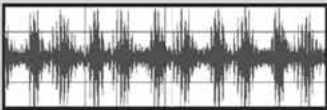
Fig. 2 Sound waveform of a scratched bearing
