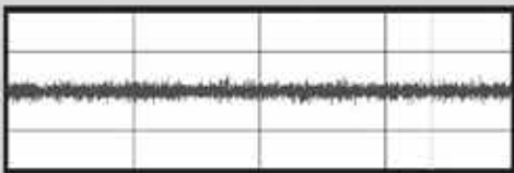
Fig. 1 Sound waveform of a normal bearing
