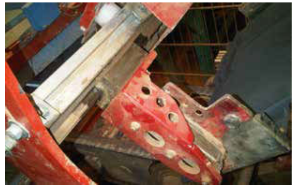
↑ Slide with solid lubrication K1 system
