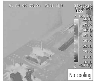
Temperature distribution without cooling
