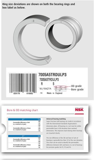
When selecting SU bearings or mixing sets of bearings to form a new or different arrangement, it is important to ensure that the bore and OD deviations are within a certain value. If the NSK sliding chart is not available, the tables shown can be used to select the maximum difference between each deviation within the set.
