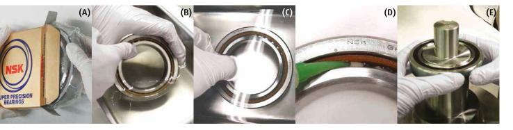
**Note:** Once bearings are washed and cleaned, avoid rotation before lubricating since this can cause damage to the rolling elements and raceways. Additional information can be found on the greasing process on page 28.
