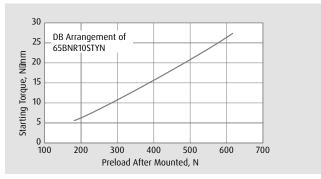
This method is best suited to applications where the preload is high. Most high-speed machine tool spindles use a lower preload and in this case the error can be large.
