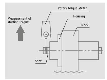
Care should be taken with this method since oil film formation in the ball contact area can cause stick – slip, this can give a higher than actual value.
