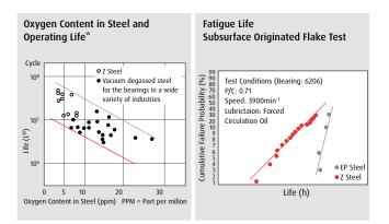
Z steel results in a fatigue life increase of 1.8 times longer than conventional Vacuum degassed steel.
