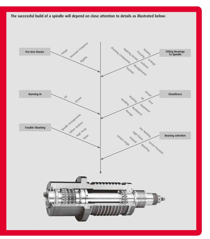
Machine Tool Precision bearings are very accurately engineered components and as such are very important to the successful performance of the machine tool. The way in which a bearing is handled and fitted to a machine tool does not only determine if the machine operates accurately but can also affect the life of the bearing in the spindle.
