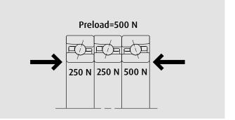
In the example of three rows, it can be seen that the internal preload is not shared evenly, this means that one bearing is taking twice the preload of the pair and will operate at a slightly higher temperature. For this reason, it can be seen from the **Speed factors table (page 18)**, that the speed capability of a set of three is less than a set of four. Load can be applied from either direction but greater load from the left side.
