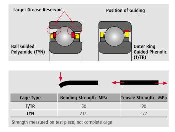
The majority of angular contact bearings use phenolic type cages and these are exceptional good for a wide range of conditions and particularly for high-speed since they are outer ring located. However, there are advantages to using TYN cages in certain applications, particularly in grease lubrication. TYN is a polyamide material and this cage is designed to be ball quided.
