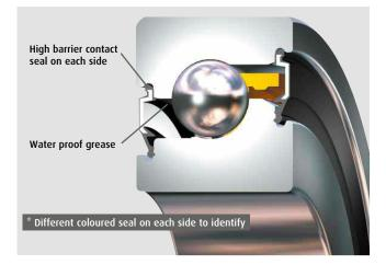
The seals are contacting type, which means that the sealing properties are excellent and each seal is a different colour to help identify the front and rear face of the bearing. A vee line is also marked on the outer ring surface for additional indication (point of vee showing front face). The grease for the sealed bearings is a special WPH waterproof type; this provides an additional barrier against water contamination.
