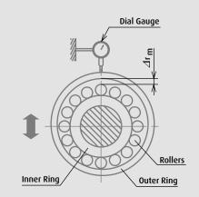
As stated on page 22 the mounted clearance of a cylindrical roller bearing is very important to the optimum performance of the spindle. When using tapered bore types it is recommended to set to a slight preload at the front of the spindle and a slight clearance to the rear of the spindle. This procedure can be easily accomplished with the use of special GN gauges (see next section).
