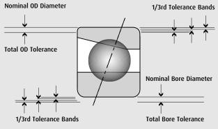
It can be seen that it would be very expensive to stock every combination of different spindle arrangements. With the use of the single micron grading the repairer only need to stock a suitable number of either SU's or DU's and the correct number of bearings can be assembled together by the repairer as long as the bore and OD deviations are within one third of the overall bearing tolerance.
