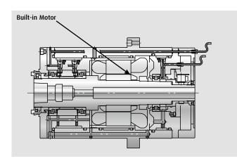
For high-speed applications using motorised spindles, the internal heat generation can be much higher than belt driven spindles; this can reduce the bearing internal clearance and sometimes cause failure at high-speed.
