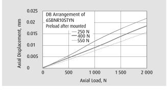
This method is better suited to lower preload applications. If the preload is very high it may be necessary to use special hydraulic equipment to apply a large enough axial load. For example if the axial rigidity is 200N/µm, an axial load of 2000N will be required to deflect the spindle by 10µm. If loads are excessive, elastically deformation can occur in both the bearing internals and associated machine parts; this could result in a measured preload being lower than actual value.
