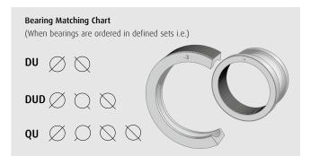
The adjacent bearings in the set are selected in the factory so that the maximum difference in bore or OD tolerance is within one third of the overall size tolerance. This is to ensure that once the bearings are fitted to the shaft and in the housing that the fits from bearing to bearing are fairly similar and thereby the load distribution within the bearing set is shared equally.
