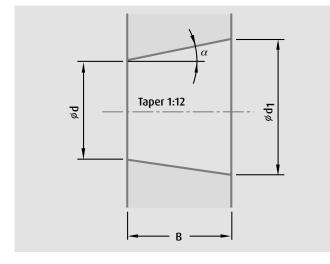
Remove the oil on the taper surface of the shaft and bore of the inner ring. Mount the inner ring assembly and place the outer ring over the rollers. Apply a dial gauge to the outer diameter of the outer ring (\*1).
