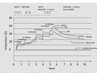
**Note:** It is very important that if the temperature of the bearings reaches 70°C, or 50°C at the housing, shut the machine down. These temperatures could cause early failure of the bearings.
