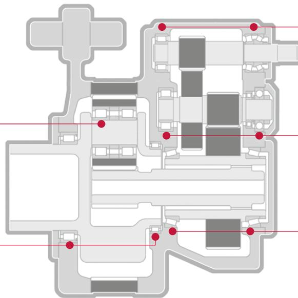
**Floating bearing** support with two **cylindrical roller bearings** NJ type. The two cylindrical roller bearings accommodate radial load and are arranged in pairs for uniform and balanced load distribution. To ensure sufficient axial clearance axial adjustment is performed by means of spacers.
