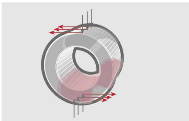
Planet gears are thin-walled machine parts exposed to high stress. On evaluating planet gear deformation, internal geometry aspects of the bearings were analysed and adjusted for uniform and balanced distribution of load. Thus improved bearing life was achieved.
