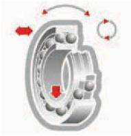
**Self Aligning Double Row Ball Bearings**
