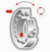
**Self Aligning Double Row Ball Bearings**
