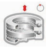
**Thrust Ball Bearings – Double Direction**
