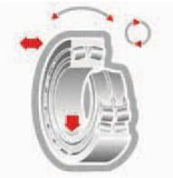
**Spherical Roller Bearings**
