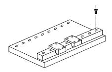
Then tighten the bolts with a torque wrench to the specified torque starting from one end.
