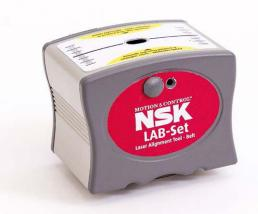
Correct alignment of belt drives is increasingly important in an environment where machine performance and maintenance costs are key considerations. Pulley misalignment can result in unnecessary forces being applied to the machinery leading to increased wear and vibration causing premature bearing failure and thereby costly machine downtime.
