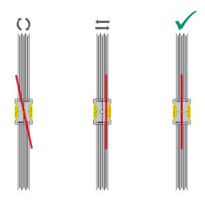
The LAB-Set units are very easily mounted on the pulleys. The spring action probe finds the centre of the belt groove. The built-in industrial magnets snap the units to the pulley in a perfect fit. Optional equipment makes it possible to align timing belt driven machines.
