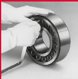
Fig. 1: Checking bearing clearance with bearing on bench.
