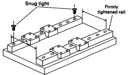
Firmly bolt the table to ball slides 1 and 2 on the firmly secured rail as shown in the diagram. Then position ball slide 3 at the left end of the adjusting rail, and bolt the table to this ball slide. Move the ball slide 3 to right and bolt the table to the ball slide 4.
