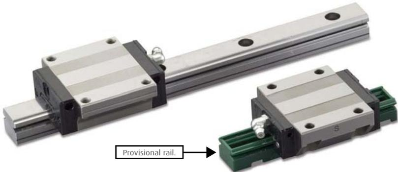
For interchangeable NH and NS Series linear guides, the ball slides and the rails are stocked separately. The ball slides are mounted on plastic provisional rails that allows for easy transfer of the ball slide to and from the steel rail.
