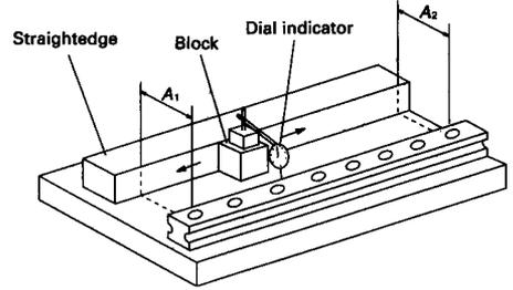
Move the dial indicator along the straightedge, and take readings at every bolt hole along the rail. Make fine adjustment of the rail to the straightedge until the desired reading is made, and tighten the bolt to the specified torque.
