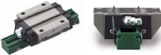
When transferring the ball slide from the provisional rail onto the rail, or vice versa, butt the provisional rail up against the rail and slide the ball slide directly from one onto the other. It is a good idea to secure the ball slide onto the provisional rail with a rubber band after removal from the rail.
