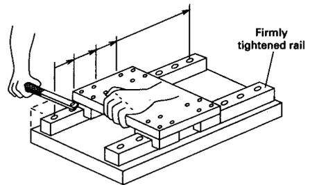
This method of assembly is for general industrial machinery where smooth linear motion is the overall objective. When precision accuracy is required, read on to the following procedure.
