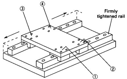
Move the table to one end of the rails, and start tightening the adjusting rail bolt sequentially to the specified torque while checking excessive friction of table movement. Continue moving the table down the rail tightening each adjacent bolt until they have all been tightened.
