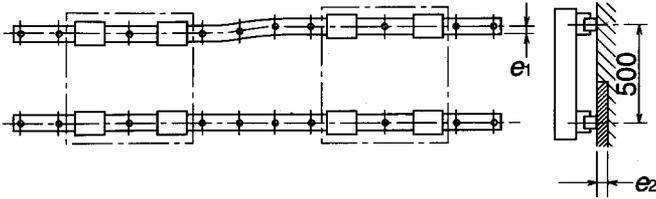
**Recommended allowable installation error of the NS Series (Maximum)**
