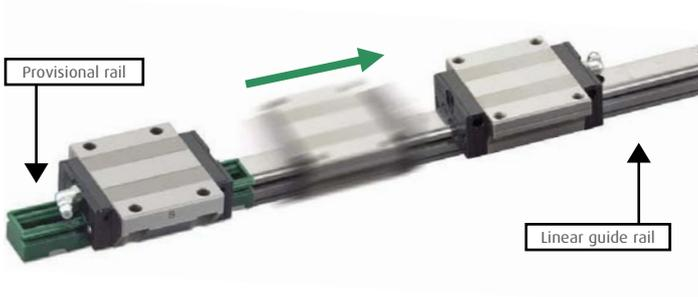
If a ball is accidentally dropped from the ball slide, it should be cleaned and replaced to the appropriate groove. The correct groove can be determined by the size of the clearance between the balls (the groove missing the ball will have greater clearance than the other grooves). It is normal to have a gap of 1.5 ball diameters in each groove.
