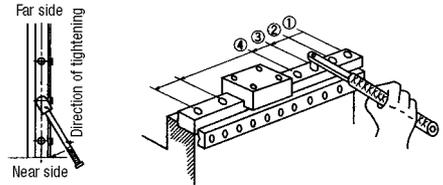
In NSK linear guides, the mounting bolt holes are processed after heat treatment using a precision machining center; therefore, the bolt hole pitch accuracy is as good as the positioning accuracy of the machine, which is considered very good.
