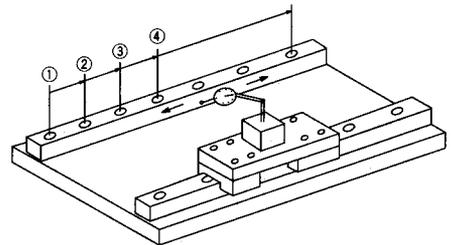
Straightness of NSK linear guides is controlled so that it can be easily adjusted manually for easy installation.
